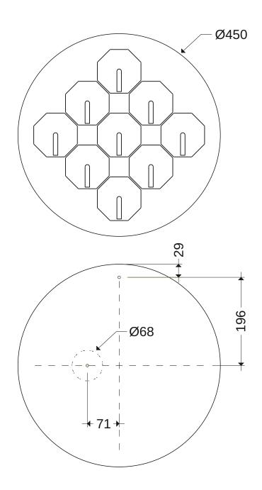
In the diagram  $\emptyset$ 68 indicates the place for a socket for concealed installation of the power supply unit in the wall.
