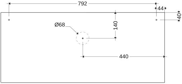
In the diagram, Ø68 indicates the location for the sub socket when the power supply is flush mounted in the wall.
